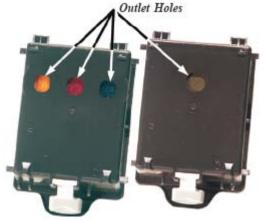
3. Push the needle all the way into the cartridge of the proper filling hole. Very slowly inject ink into the sponge until the cartridge is full. Approximately 5-6 ml per chamber. (This will saturate the sponge with ink).
